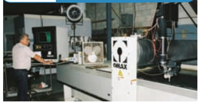
Diamond F.C. is using the Omax JetMachining Center that the firm recently installed to cut a variety of materials including stainless steel, aluminum, glass, plastics, and more.
